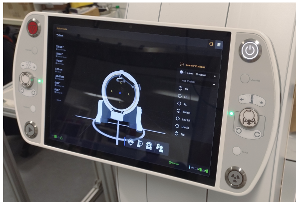
Figure 2.3.: Control Panel with Movement Controls on the Right, Detector Position and Start/Stop for Preprogrammed Movements on the Left
